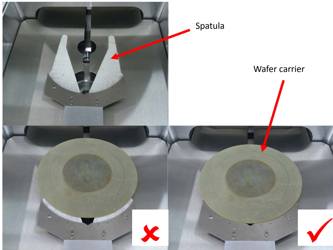
Fig. 4: Position of the wafer carrier on the white spatula
