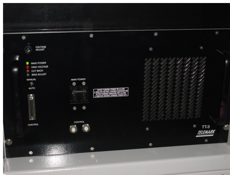
Fig 4: TELEMARK TT-3 High Voltage DC Power Supply
